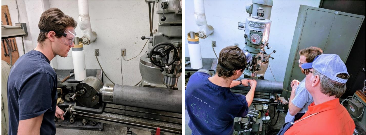
Figure 15: Safety Officer Drew Ross milling out the fin slots (left), Team Lead Stefan Tomovic and Drew Ross aligning the mill with the body tube (right)
