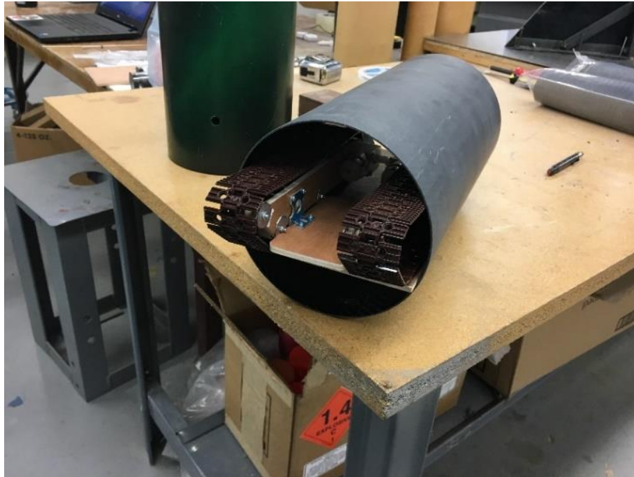
Figure 58: Rover inside Rover Deployment System coupler
