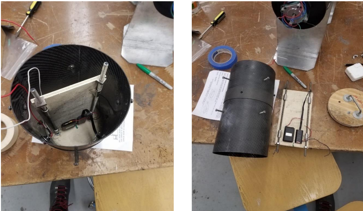
Figure 17: Avionics Bay sled in coupler (left) avionics bay coupler and sled disassembled (right)
