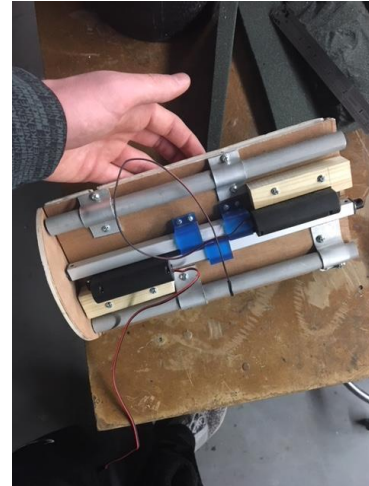
Figure 67: 3D model of base plate and linear actuator (left), constructed base plate and linear actuators (right)
