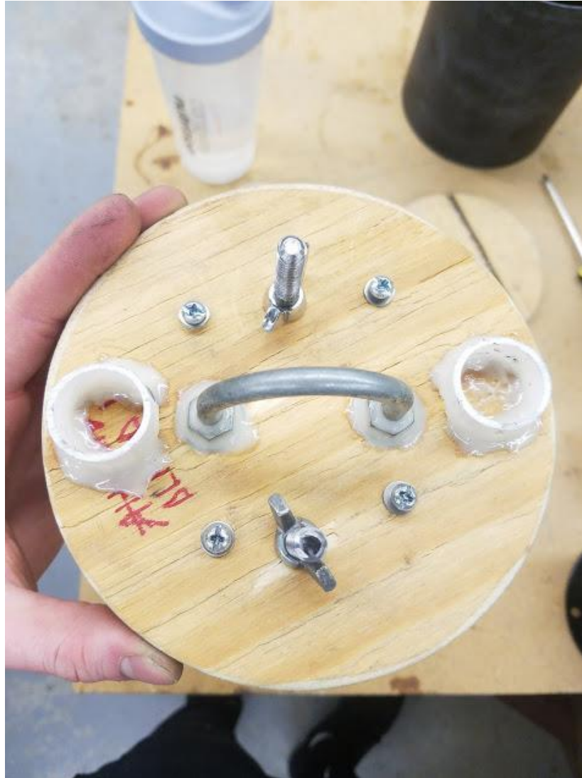
Figure 26: Fore bulkhead of altimeter bay. PVC piping for holding the charges can be seen, along with U-bolt for the main parachute, and the small bolts for the e-matches to connect to the altimeter
