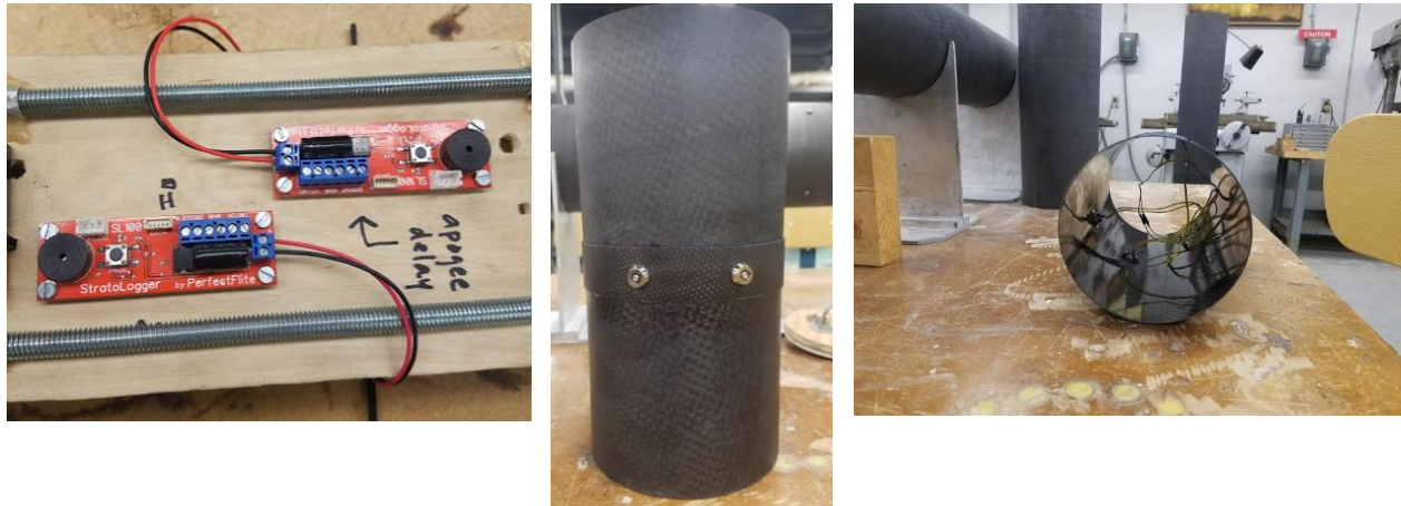
Figure 27: PerfectFlite SL100 Altimeters (left), key switches (middle), wiring of switches (right)
