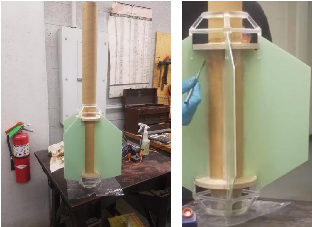
Figure 14: Fin Jig Mk2 implemented on inner tube with fins aligned
